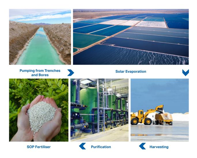
Figure 8.2: A visual representation of the production of a solar evaporation SOP project.
